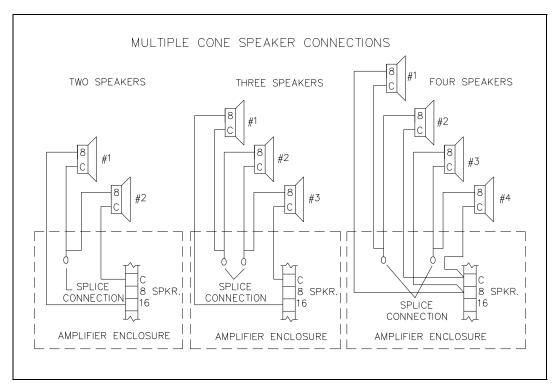
Figure 1. Cone Speaker Connections
