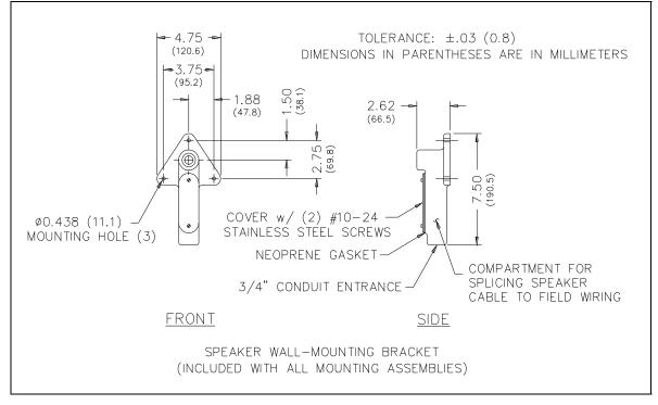
Figure 3. Wall Mounting Bracket
