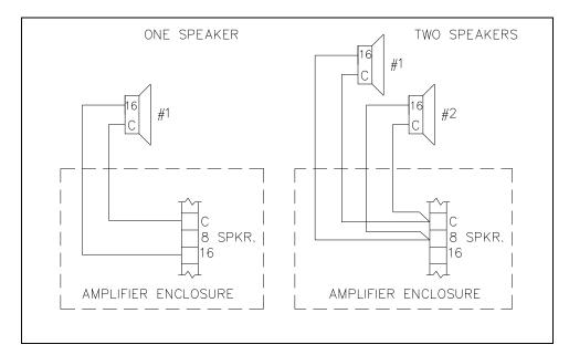
Figure 2. 16-ohm Speaker Connections
